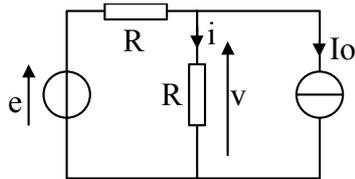
$$\left. \begin{array}{l} e(t) = R \cdot i(t) + R \cdot (i(t) + I_o) \\ v(t) = R \cdot i(t) \end{array} \right\} \Rightarrow i(t) = \frac{e(t) - R \cdot I_o}{2 \cdot R} \Rightarrow v(t) = \frac{e(t) - R \cdot I_o}{2} = 5 \cdot \cos(\omega t) - 5$$
