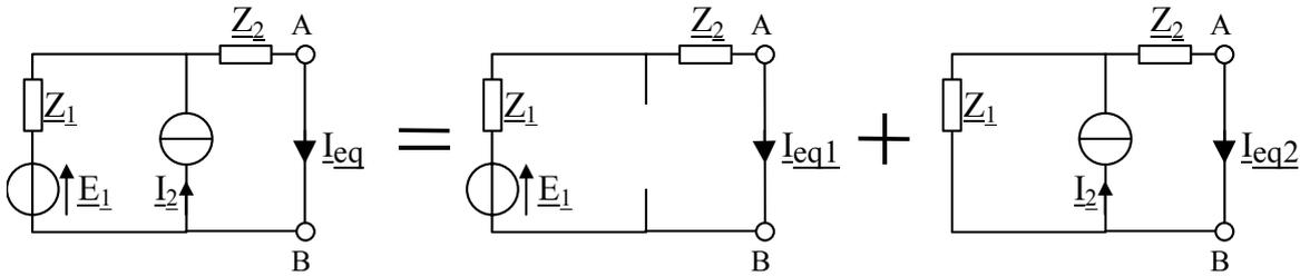
$$\underline{I_{eq}} = \underline{I_{eq1}} + \underline{I_{eq2}} = \frac{\underline{E_1}}{\underline{Z_1} + \underline{Z_2}} + \frac{\underline{I_2} \cdot \underline{Z_1}}{\underline{Z_1} + \underline{Z_2}} = \frac{\underline{E_1} + \underline{I_2} \cdot \underline{Z_1}}{\underline{Z_1} + \underline{Z_2}}$$
