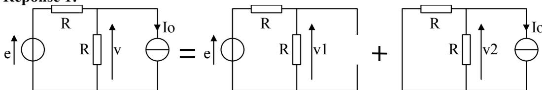
$$v_1(t) = \frac{e_1(t)}{2} \quad v_2(t) = -\frac{R}{2} \cdot I_o \quad \Rightarrow v(t) = 5 \cdot \cos(\omega t) - 5$$
