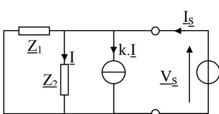
$$\underline{I} = \frac{V_s}{\underline{Z}_2} \quad \cdot \quad \underline{I}_s = \frac{V_s}{\underline{Z}_1} + (1 + k) \cdot \underline{I} = \frac{V_s}{\underline{Z}_1} + (1 + k) \cdot \frac{V_s}{\underline{Z}_2}$$
