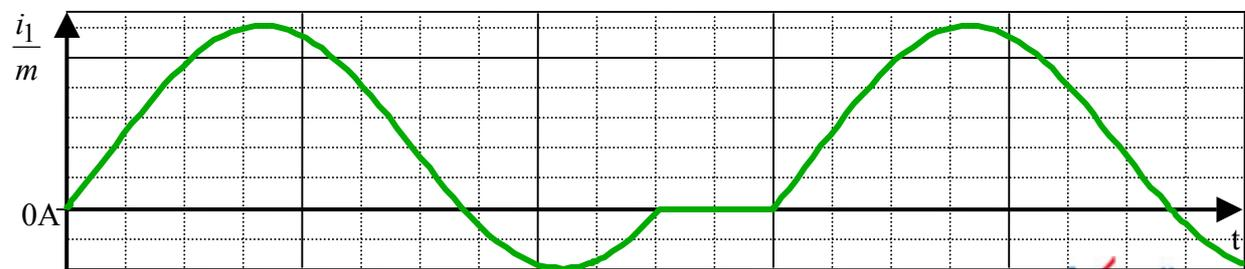
$$\mathbf{c1)} \omega_o = \frac{1}{\sqrt{L_o.C_o}} \Leftrightarrow f_o = \frac{\omega_o}{2.\pi} = \frac{1}{2.\pi.\sqrt{L_o.C_o}} \Leftrightarrow [t_0, t_3] = \frac{1}{f_o} = 2.\pi.\sqrt{L_o.C_o}$$
