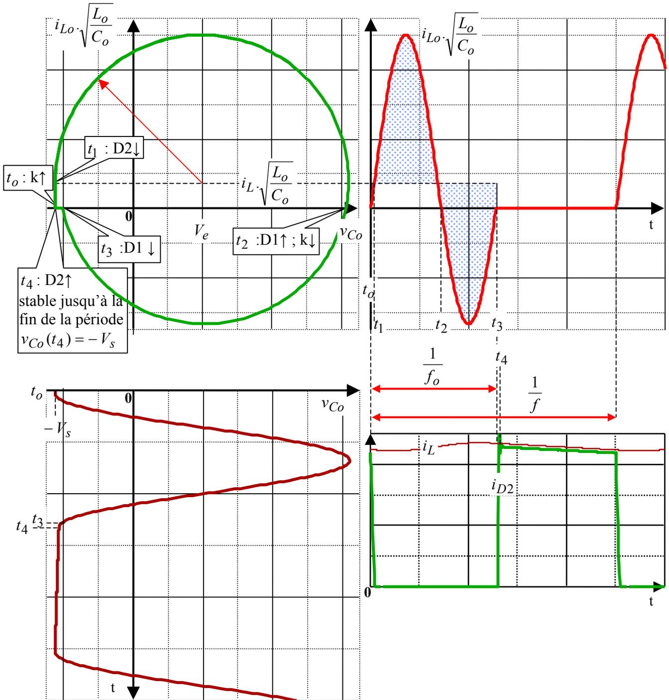
c1)  $\omega_o = \frac{1}{\sqrt{L_o \cdot C_o}} \Leftrightarrow f_o = \frac{\omega_o}{2\pi} = \frac{1}{2\pi \cdot \sqrt{L_o \cdot C_o}} \Leftrightarrow [t_o, t_3] = \frac{1}{f_o} = 2\pi \cdot \sqrt{L_o \cdot C_o}$
