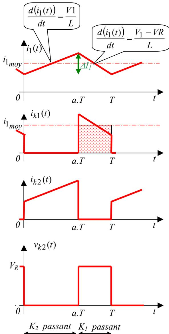
$$\left. \begin{array}{l} k2 \text{ conduit} \\ k1 \text{ ouvert} \end{array} \right\} \Rightarrow V_1 = L \cdot \frac{d(i_1(t))}{dt} \Leftrightarrow \frac{d(i_1(t))}{dt} = \frac{V_1}{L} > 0$$
