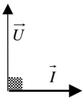
Donc  $Q_L = U_{eff} \cdot I_{eff} \cdot \sin(\varphi) \Rightarrow Q_L = L \cdot \omega \cdot I_{eff}^2 = \frac{U_{eff}^2}{L \cdot \omega} = U_{eff} \cdot I_{eff}$
