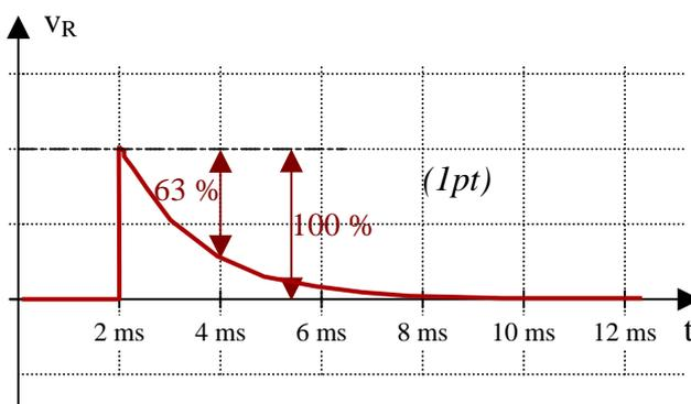
$$v_C(t) = (0 - E).e^{-\frac{t-t_0}{R.C}} + E \quad (1pt); \quad v_R(t) = (E).e^{-\frac{t-t_0}{R.C}} \quad (1pt)$$
